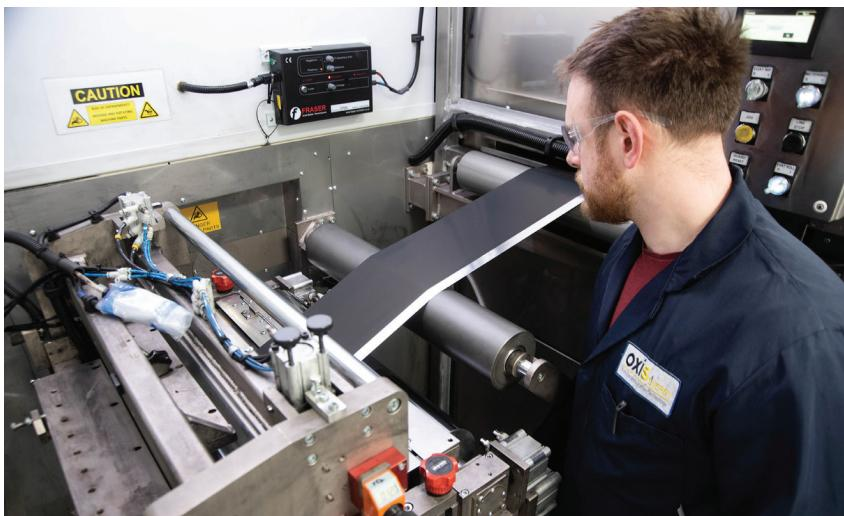
**ALL AMPED UP:** Bye Aerospace's eFlyer 2 [top] is designed to train pilots. Bye is working with Oxis Energy on a lithium-sulfur battery that promises to increase the plane's range. Here a reel of positive electrode, made of sulfur, is being coated onto a current collector [bottom].
